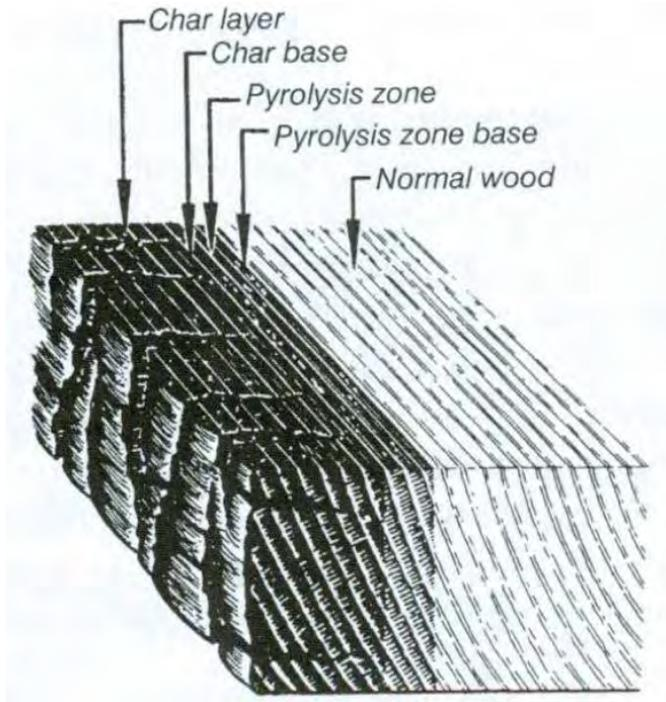
The char layer grows with sustained exposure to fire, creating even more insulation, slowing down the burning rate and reducing the unheated cross section of the member (AITC, 2012). This behavior continues until the end of heating, or the section has completely combusted.
