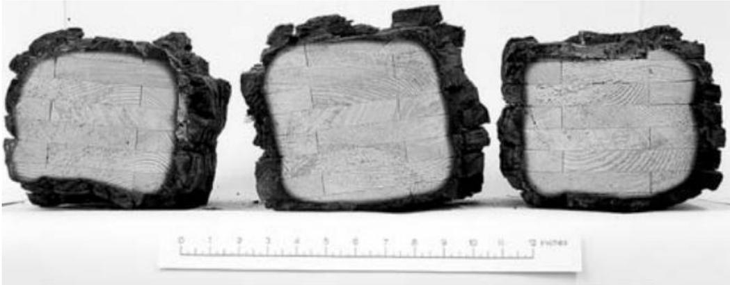
Fire performance of heavy timber sections is demonstrated in the image below, showing floor framing after a fire. The panel above the floor framing has burnt away, but the heavy timber members have survived the fire.
