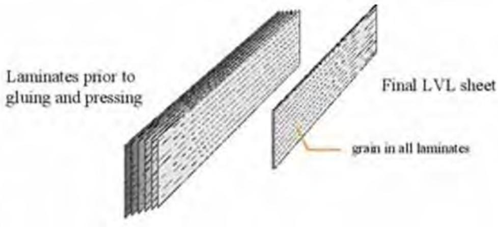
Figure 22 – LVL elements (Green, The Case For Tall Wood Buildings, 2012)
