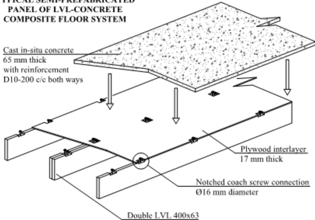
Figure 48 – Rendering of timber-concrete composite floors in a multi-story post and beam building application (Rhomberg, Life Cycle Tower, 2012)
