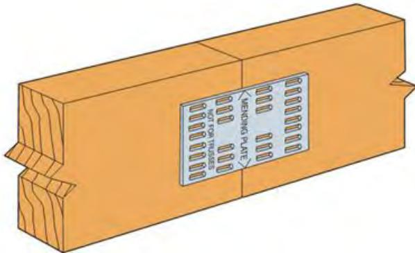
Figure 18 – Example of truss plate frames (Drang, 2010)
