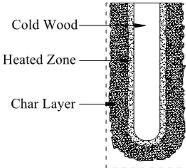
The section of timber in the heated zone beyond the char layer is known as the pyrolysis zone, and corresponds to temperatures between approximately 392°F [200°C] and 572°F [300°C] (AWC, Calculating the Fire Resistance of Exposed Wood Members, 2003). Within this zone, timber is assumed to undergo thermal decomposition and pyrolysis.
