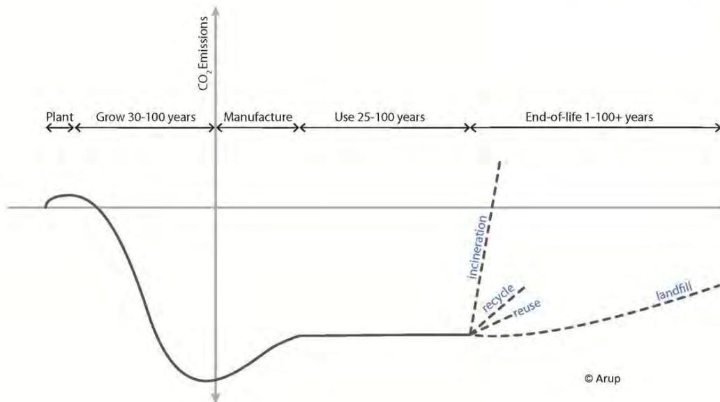
At the beginning there is a relatively small amount of carbon emitted, assuming some human activity in fostering tree growth. During growth the greatest amount of carbon is absorbed, shown by the dip in the graph. In harvesting and manufacture, some carbon is emitted again, but not nearly as much as has been absorbed if the tree was allowed to grow throughout the time it could absorb carbon at its highest rate.
