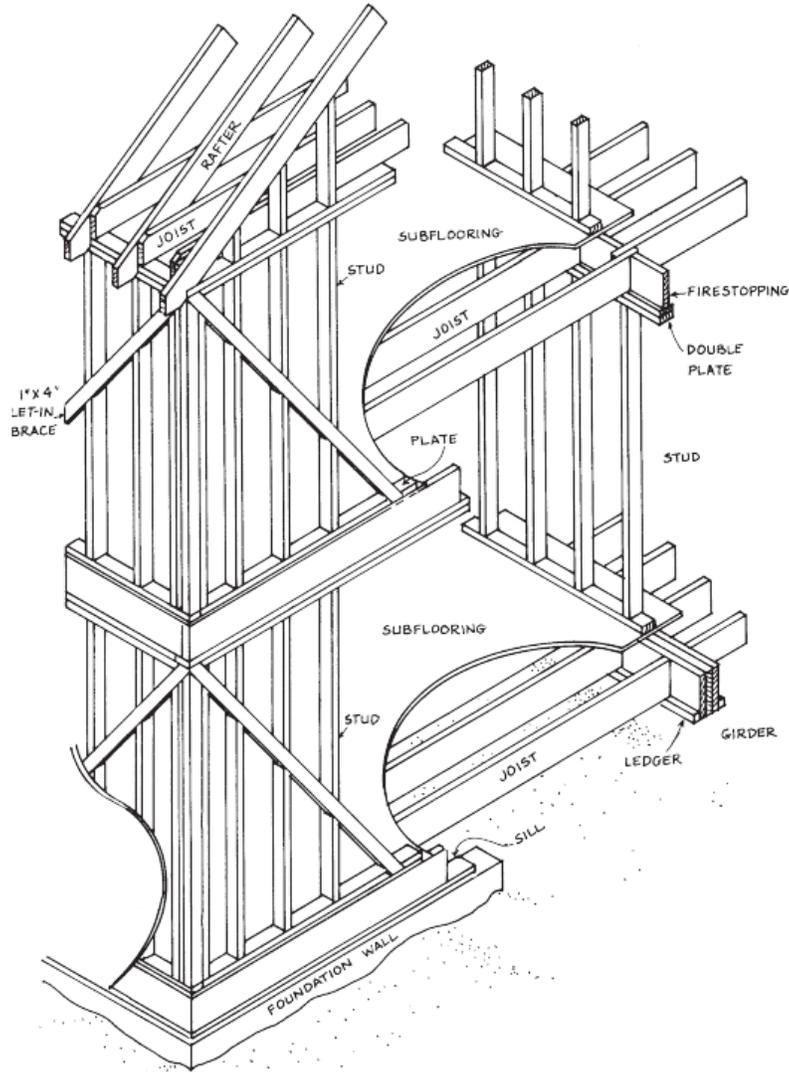
Figure 9 – Typical balloon-framing (AFPA, 2001)
