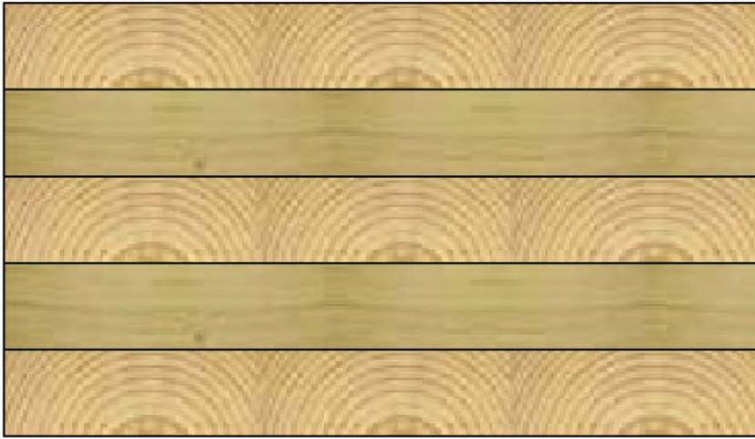
Figure 25 – Example of a 5-layer CLT panel showing layer orientation (FPInnovations, Cross Laminated Timber (CLT), 2013)
