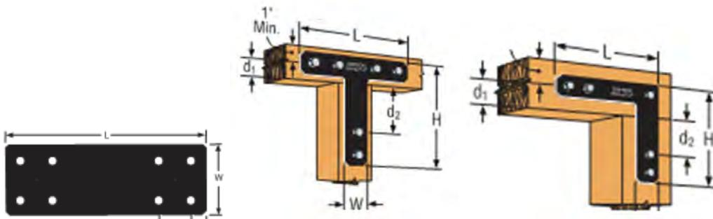
Examples of embedded steel plate connections in heavy timber are shown in the image below.
