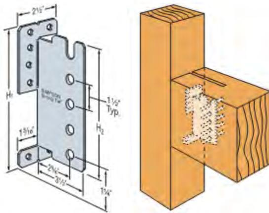
Plates can also be embedded in panelized construction. While these plates are thicker than plates in light timber frames, they often still utilize screws to fix the connector in place (Gagnon & Pirvu, 2011).
