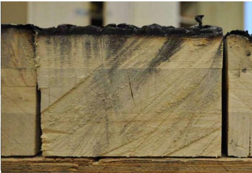
Figure 61 – CLT member showing charring depth on a wall member (Osborne, Dagenais, & Benichou, 2012)
