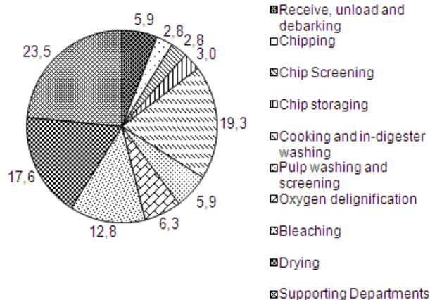
**Figure 4.** A case of cost distribution in a kraft Scots pine pulpmill (Korpunen et al 2010b).
