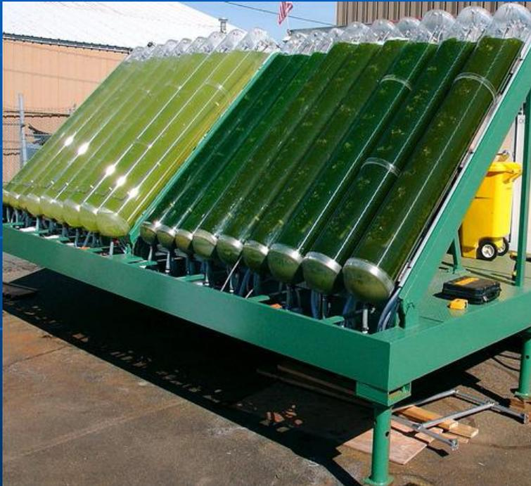
A Photo-Bioreactor in Translucent Tube from GreenFuels
