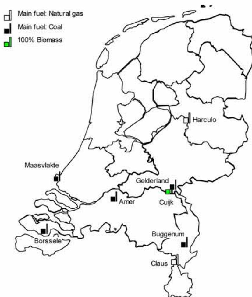
Figure 5. Overview of all plants in the Netherlands with a biomass (co-)firing capacity of over 20 MW e in 2005. Source; www.energie.nl .
